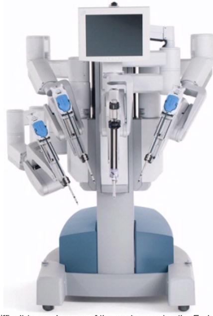
Robot-assisted surgery offers surgeons greater access to difficult-to-reach areas of the anatomy using the EndoWrist instruments. Robotic technology seamlessly translates the surgeon's movements into precise, real-time movements of the surgical instruments.
